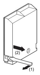
• Lift cover and remove screw from cable clamp.
